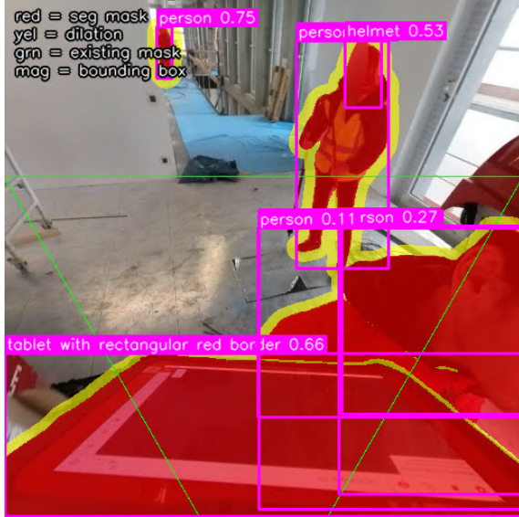
Figure 6. Carrier masking on a virtual perspective view. YOLOE detects the person, helmet, and tablet; the segmentation mask (red) is dilated (yellow) before being unioned with a static carrier template (green) to suppress feature observations on the operator.
